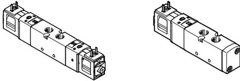
In-line valve VUVS-LT as individual valve (disc seat valve)
