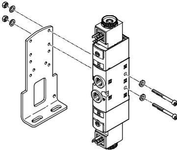
For mounting individual valves on a flat surface, e.g. aluminium profile systems.
