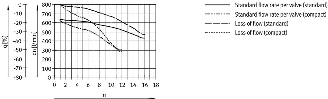
For 5/2-way valves, valve manifold
