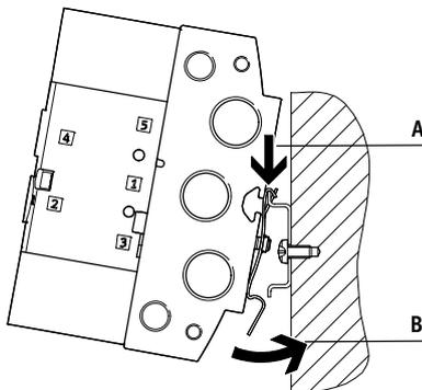
The H-rail mounting VAME-T-M... consists of two mounting clips. These are screwed to the manifold block on the left and right.
