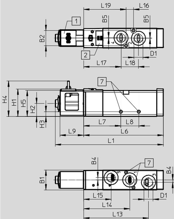
1 Solenoid coil interface type C    2 Location for inscription label    7 For screw M3
