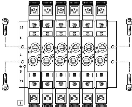
Sturdy wall mounting of the manifold block using four through-holes.
