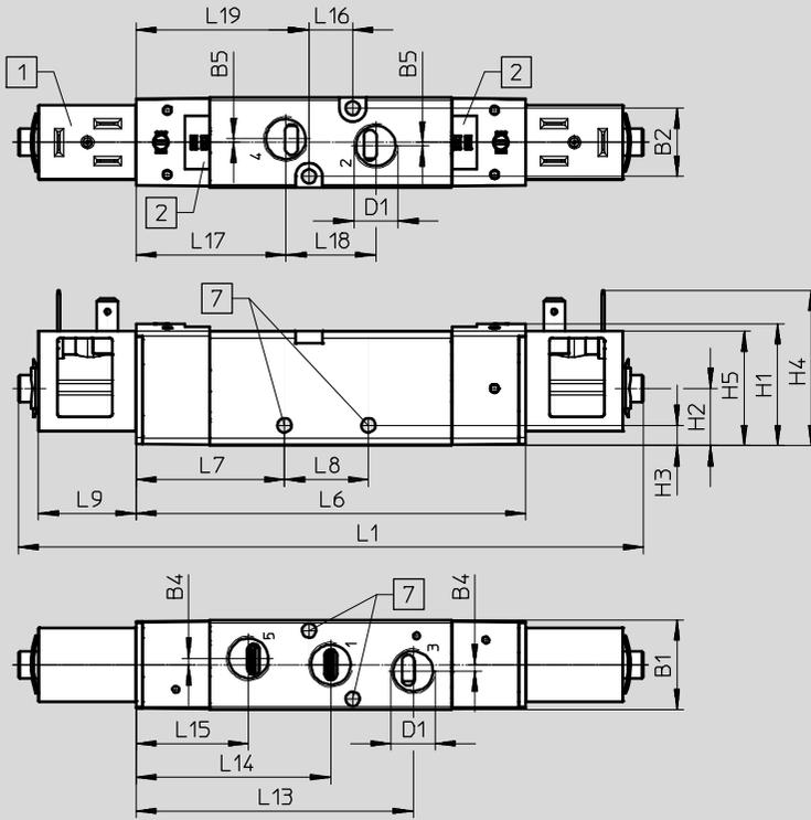
1 Solenoid coil interface type B      2 Location for inscription label      7 For screw M4
